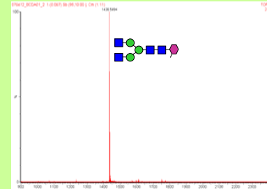
Figure 1. Mass spectrometric (MALDI-TOF) analysis of N-glycans labeled with 2-AA released from LEX Opt Rituximab. Structures are illustrated using the symbol nomenclature outlined by the Consortium for Functional Glycomics ( http://www.functionalglycomics.org ).
